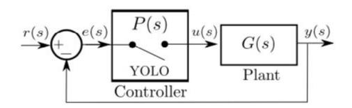
$$F_{inactive}(s) = \frac{y(s)}{r(s)} = \frac{P(s)G(s)}{1 + P(s)G(s)} \qquad \qquad F_{active}(s) = \frac{y(s)}{u(s)} = G(s)$$
