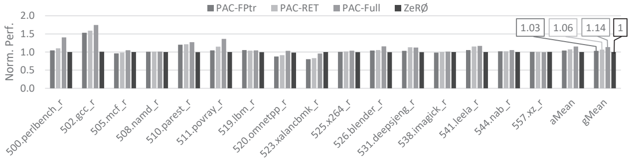
Fig. 8: Performance overheads of ZeR0 and three different ARM PAC configurations for the SPEC CPU2017 benchmark suite.
