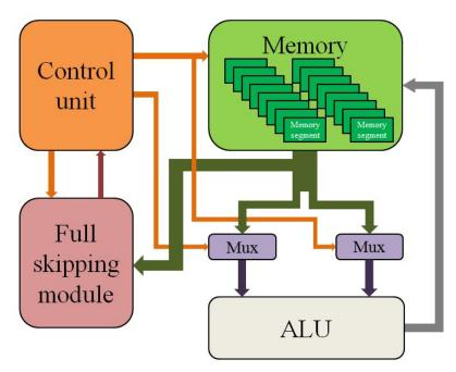
FIGURE 4.3: The architecture for Gaussian with full skipping.
