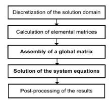
FIGURE B.1: Flow chart for the finite element algorithm.
