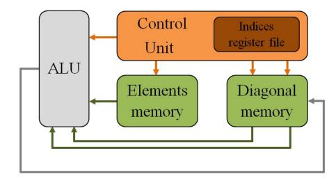
FIGURE 4.5: The architecture for Gaussian using sparse model.
