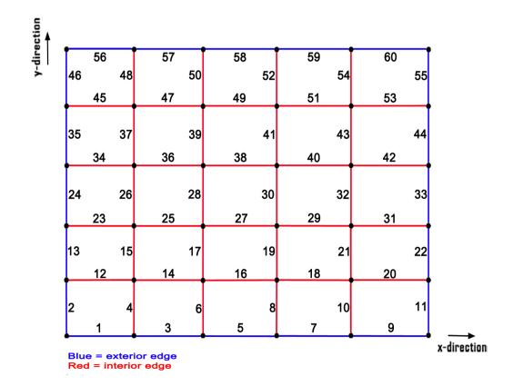
FIGURE 6.6: Using interior edges only from mesh grid.
