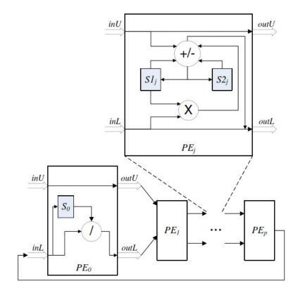
FIGURE 2.1: LU Factorization Design Block Diagram.
