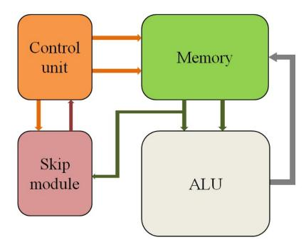
FIGURE 4.2: The architecture for Gaussian with skip.
