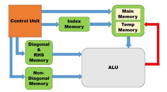
FIGURE 5.1: The architecture for Basic Jacobi.
