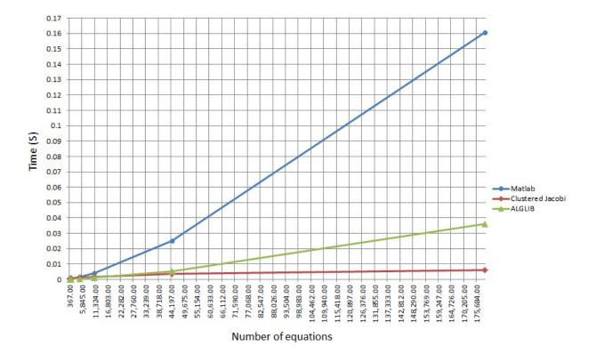
FIGURE 7.4: 32 bit Floating-point Clustered Jacobi Hardware vs Software
