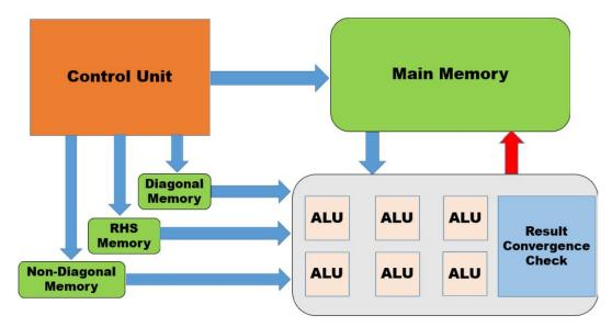
FIGURE 5.4: The architecture for Clustered Jacobi.
