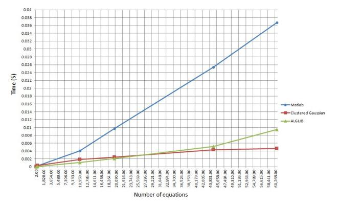
FIGURE 7.3: 32 bit Floating-point Clustered Gaussian Hardware vs Software
