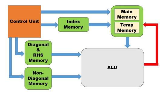
FIGURE 5.3: The architecture for Pipelined Jacobi.
