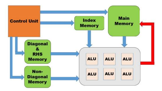
FIGURE 5.2: The architecture for Parallel Jacobi.
